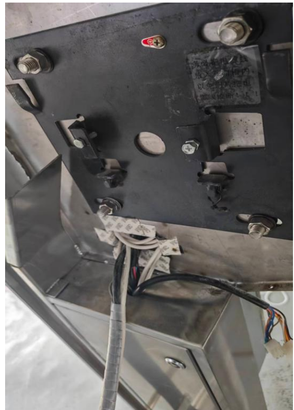
Figure 6. Drive-shaft mounting area at the top of a side post.
