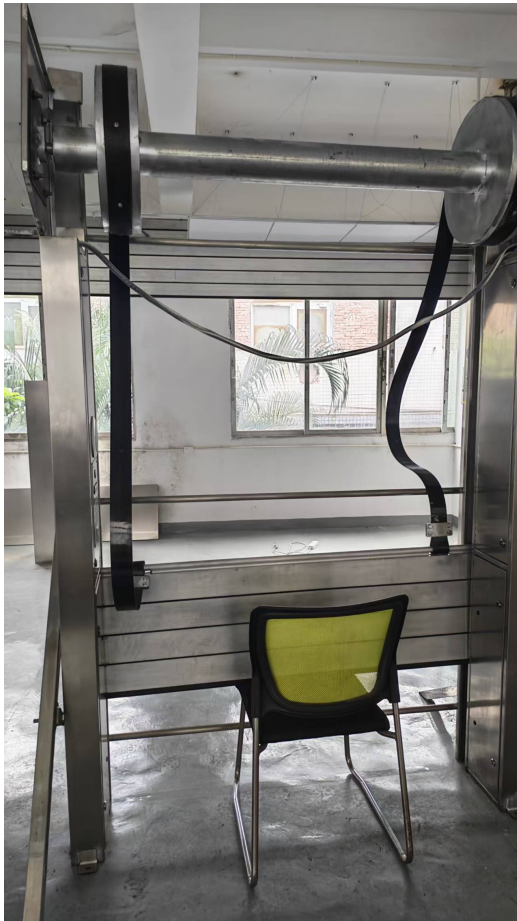
Figure 7. Drive shaft installed across the top of the gate.
