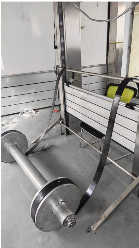
Figure 5. Drive shaft and steel straps before the shaft is lifted into position.
